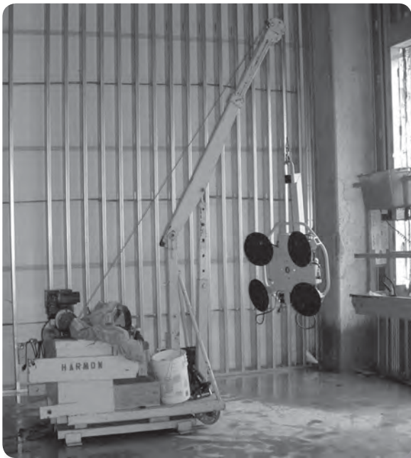
Power vacuum lifter avoids manual lifting
