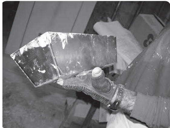
Solution: Holding mud pan with glove
