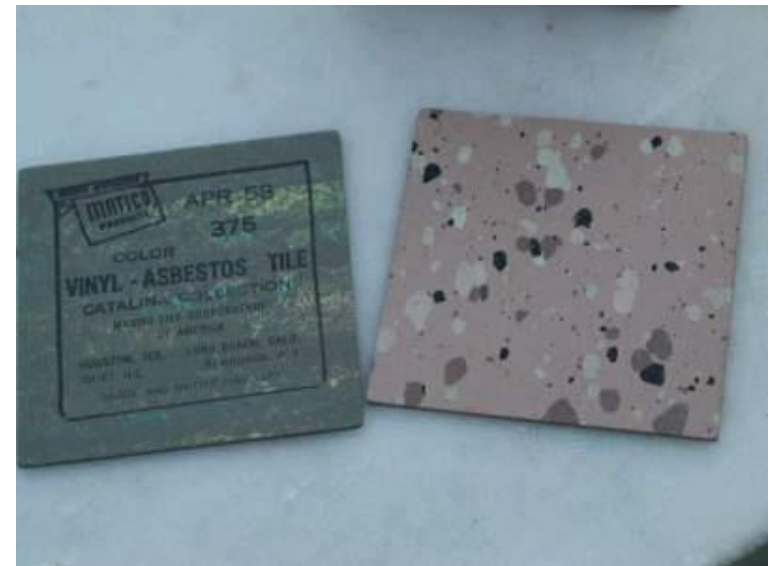
Vinyl asbestos flooring
